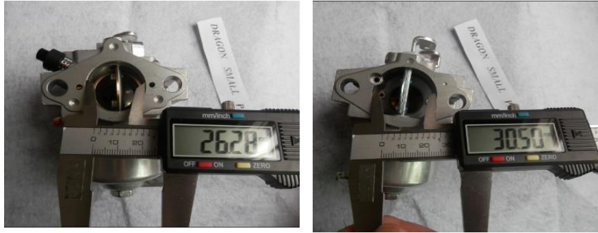
Figure 3.4: Base engine carburetor dimensions from online retailer
